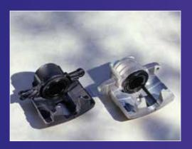
Metal matrix composite brake calipers employing Nextel ceramic textiles are half the weight of steel or cast iron, but with equal or better strength and stiffness.
