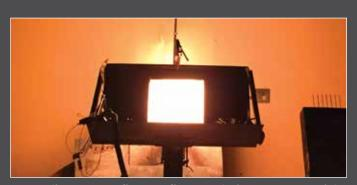
According to FAA fireproofing regulations, commercial engine cowlings must be capable of withstanding a flame of 2000°F (1093°C) for 15 minutes without flame penetration. Nextel ceramic textiles help manufacturers exceed this requirement.
