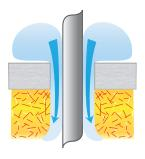
A draft fan  $\Delta P$  of 0.35" of water draws outside air through a nominal 1 ft² gap at a rate of 1.92 lbs/sec., every day, every month, every year. Tube seals made using Nextel ceramic textiles help stop the ingress of air.
