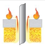
The temperatures inside a process heater can reach 2000°F and above. In instances of draft fan failures, this heat may cause extreme damage to a furnace penthouse. Nextel fiber can withstand direct flame impingement and prevent flame penetration.
