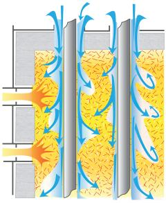
Tube seals are designed to stop the ingress of cold air into a furnace heater box. Draft fan induced, negative pressure process heaters, such as steam methane reformers, ethylene heaters and ammonia reformers, draw in air through the openings around each tube penetration. This cold air is an added load. The money spent heating this may be recovered in less than six months with the successful installation of a tube seal made using Nextel ceramic textiles.
