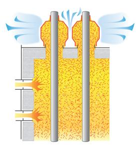
This is a process heater outfitted with tube seals made using 3M™ Nextel™ Ceramic Textiles. They prevent the ingress of tramp air and save money by decreasing fuel consumption, reducing heat losses and controlling excess oxygen.
