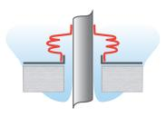
Tube seals are designed to flex to allow for the expansion of the process tube relative to the furnace roof. Tube seals made using Nextel ceramic textiles remain flexible for years of continuous operation up to 2200°F.
