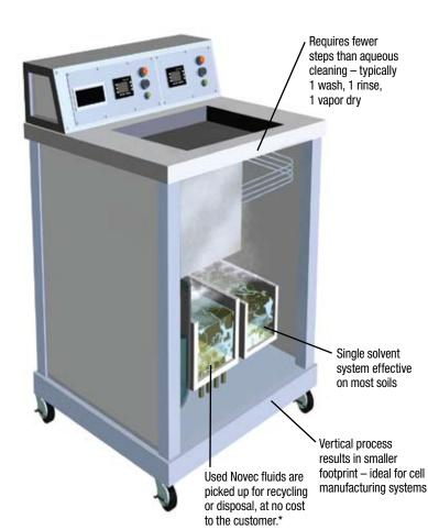
Solvent Cleaning with 3M<sup>™</sup> Novec<sup>™</sup> Engineered Fluids
