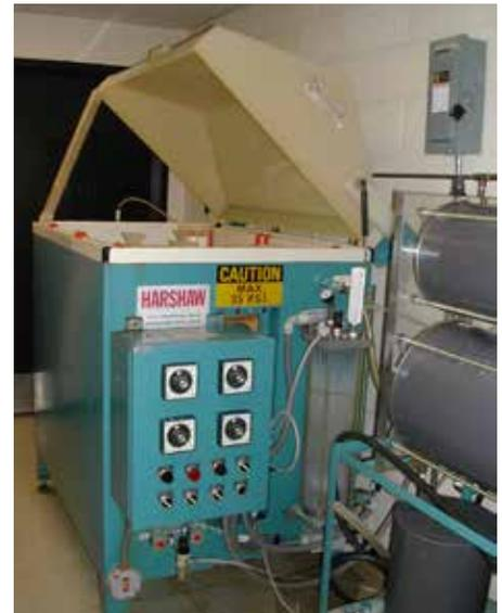
Figure 2. Specimens in this experiment were exposed in the Harshaw salt spray (fog) unit shown above.
