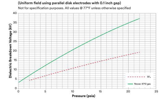
Dielectric Breakdown Voltage of Novec 4710 Gas Compared to SF<sub>6</sub>
