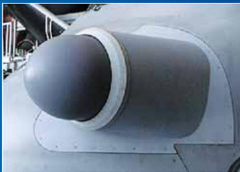
Because of their electromagnetic transparency, PMCs made with Nextel ceramic fibers are ideal for applications such as aircraft radomes.
