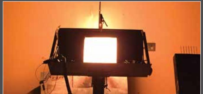
According to FAA fireproofing regulations, commercial engine cowlings must be capable of withstanding a flame of 2000°F (1093°C) for 15 minutes without flame penetration. Nextel ceramic textiles help manufacturers exceed this requirement.
